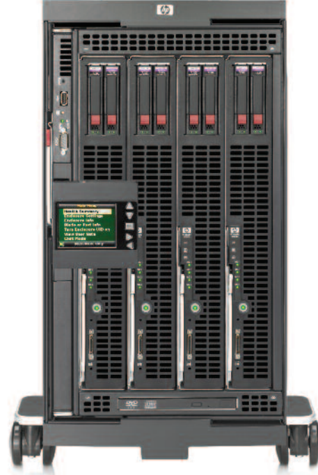
HP c3000 tower enclosure with Onboard Administrator module and HP BL860c server blades
